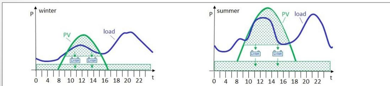
Fig. 11: Load curve and supply scheme for application geographical island
