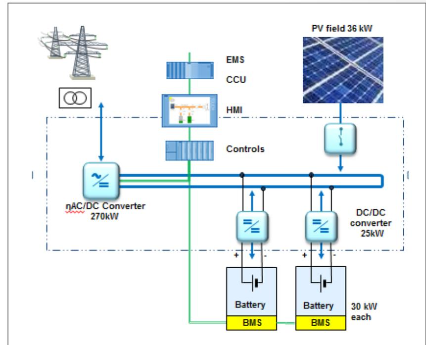
Fig. 10: Schematic system overview
