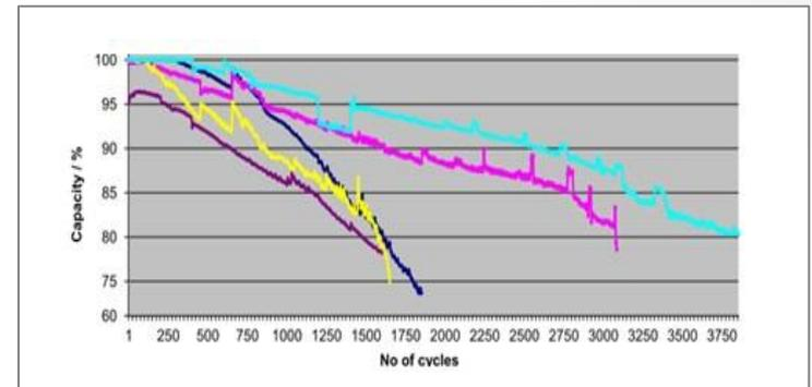
Fig. 3: Cycle trend of different Li ion batteries
