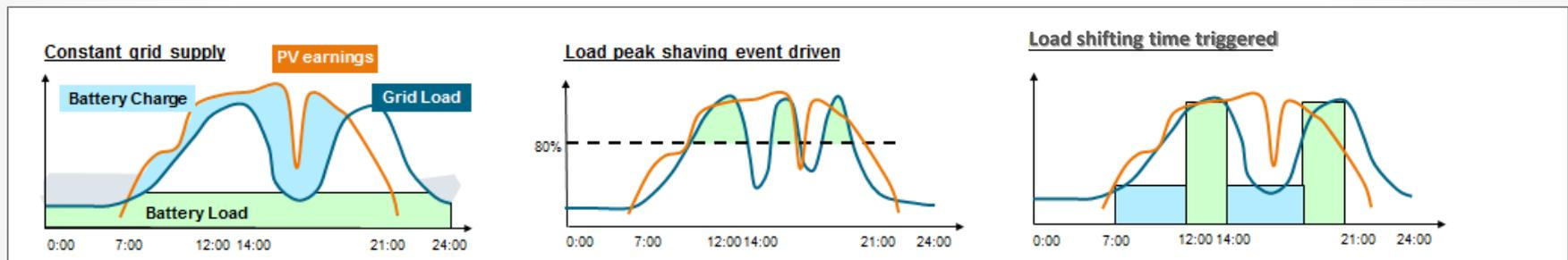
Fig. 1: Required operation modes for an Electrical Energy Storage system (EES)
